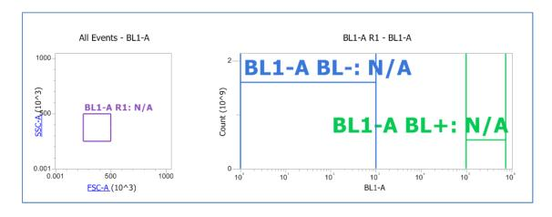
10. Load Tube 1 and click RUN. Open Instrument settings -> Voltage tab. Adjust the FSC and SSC voltages until the beads are on scale (the values in the picture are not accurate). Click STOP.
