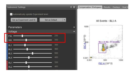
11. Shift the gate to include the bead population, excluding the multimers. See the plot below for an example. Right click on the gate to Apply gate shape to all controls.
