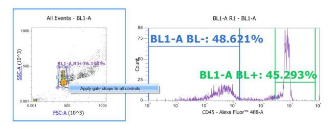
12. Click Run again and adjust the voltage of BL1 channel so that the negative beads are around  $10^2$ - $10^3$  region, making sure that the positively stained beads are within scale (see image above).
